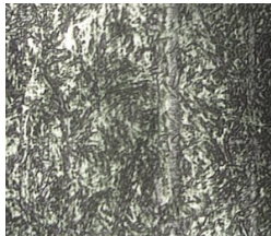
Gambar 14. Struktur Mikro hasil quench media air temperatur 26°C, perbesaran 2000x
